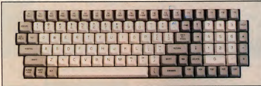
The keyboard has 105 full-stroke keys. The top and bottom rows contain 24 programmable function keys.
